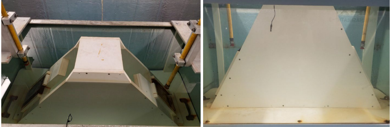
Figure C- 2. Top view (left) and side view (right) of submerged jet test set-up.
