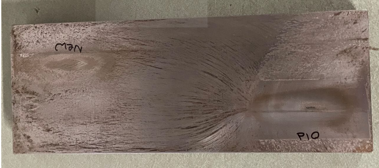
Figure C- 6. Photo of mild steel after 40-hrs of cavitation testing.
